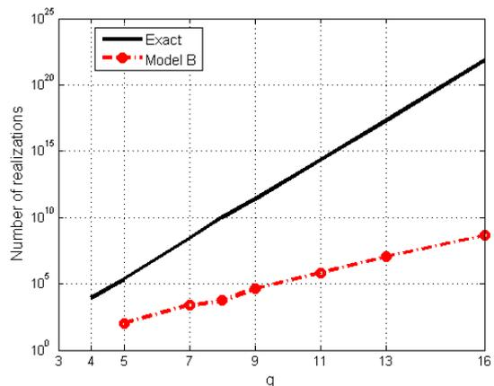
Fig. 4: The number of realizations required for evaluating  $P_m$  for  $M > q/2$ . This number is zero for all  $q$  in the case of Model A.
