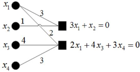
Fig. 1: Example for a Tanner graph (over  $\text{GF}(5)$ ). Circles denote variable nodes, and squares denote check nodes.
