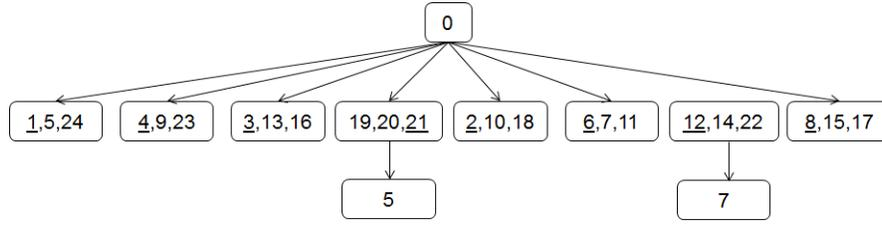
Fig. 6. Example of decoding a request with burst length 9, where  $T = \{1, 2, \dots, 8\}$  are unrequested elements. The element requested with multiplicity is the root of the tree 0. The underlined element in each child of 0 is a systematic helper used to solve 0. For the children sets  $\{19, 20, 21\}$  and  $\{12, 14, 22\}$ , all elements are requested, and therefore the chosen systematic helpers 21 and 12 need 5 and 7, respectively, as their helpers.
