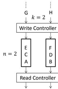
Fig. 2. Packet placement in a memory system for  $k = 2$  input/output packets, with  $n = 2$  memory banks. 2 banks are *not* sufficient to allow reading any 2 packets without contention.
